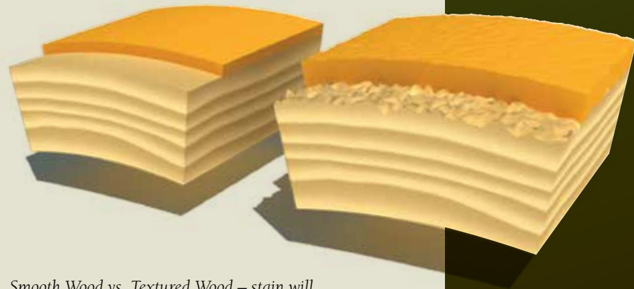
Smooth Wood vs. Textured Wood – stain will adhere much better to the textured wood on the right, improving performance and longevity.
