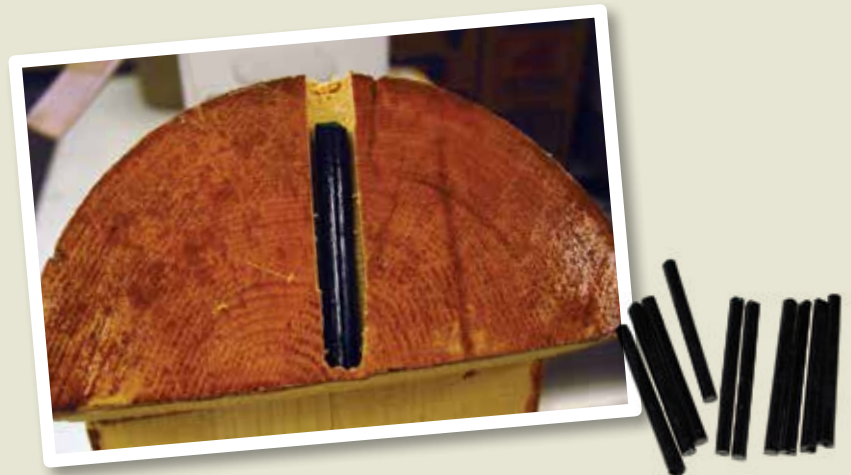
Log cross-section showing an installed borate rod.
